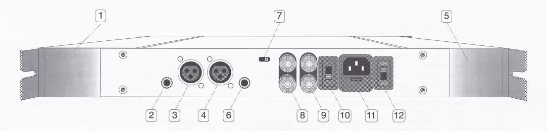
1: Cooling Duct Exhaust
