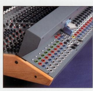
The meter bridge is capable of folding flat for shipping and is easily pivoted forward for operation. A ribbon cable connects the meter bridge to the body of the Remix.
